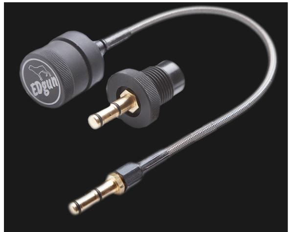
Important: While filling the gun with the high pressure pumps (like Hill pump) you should make few quick and powerful movements of the pump handle to increase the pressure in the filling hose in order to “raise up” the O-rings on the filling probe, otherwise there will be leakage of the air and you will not be able to fill the gun.
