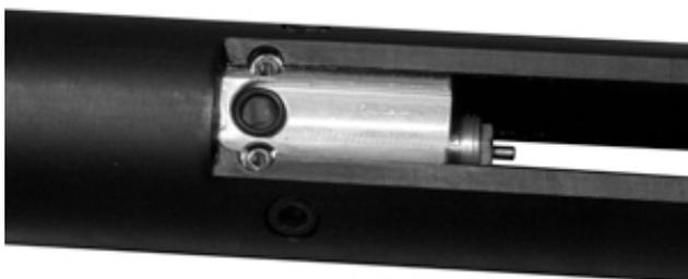
The breech installing together with the sliding bar and the plate to keep it together you should cover it with your hand keeping your fingers at the plate to avoid it to fall from the breech. Then push the breech to the breechring.
