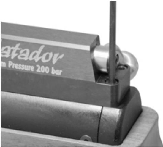
Move the breech backward until it is taken off the gun. Be sure to keep the sliding bar and its plate with your fingers while taking the breech off not to lost it.
