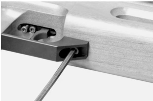
Remove the trigger bracket from the gunstock.
